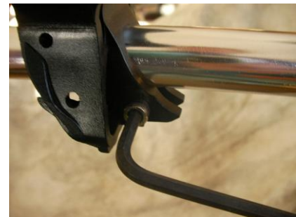
Loosen the screw in the bottom of the heel to adjust length.
