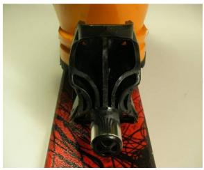
Once the heel throw is in the correct length position, align it vertically and tighten the bracket screw.
