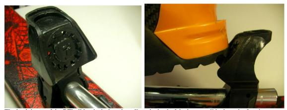
The heel throw of the RTbulldog is designed to allow the heel of the boot to slide down its face into a seated position. The spring inside the tube allows the throw to slide back with downward pressure from the heel of the boot.
